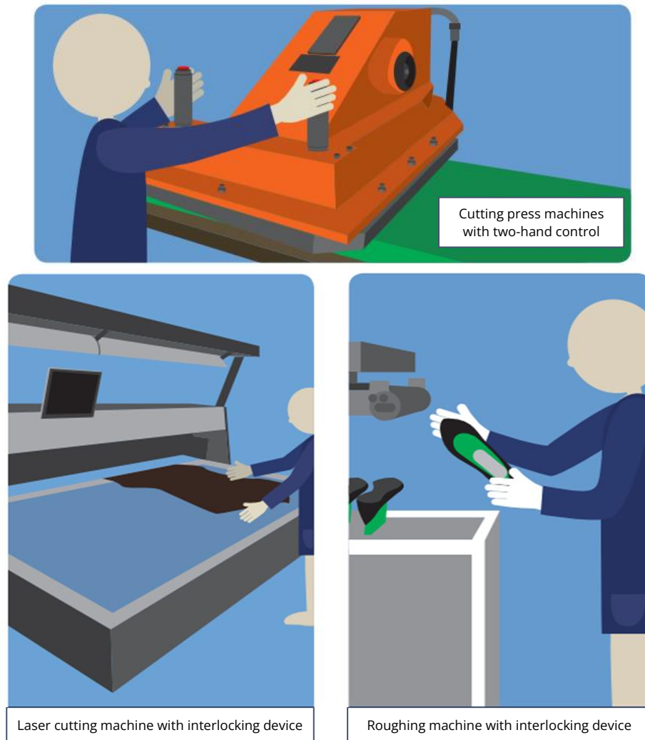
Fig. 14: Mechanical risks and prevention in footwear manufacturing. Source: Preventing mechanical risks, ACT
