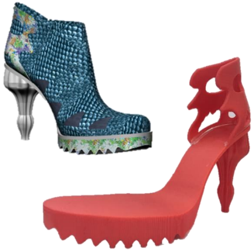
Fig. 4: 3D printed prototypes of footwear components. Source: TUIASI
