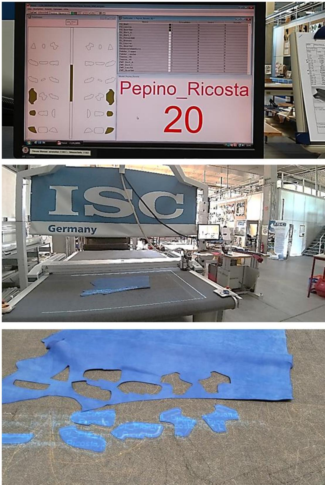
Fig. 5: Automatic cutting table
