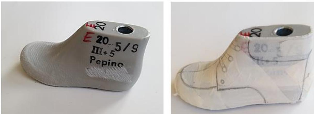
Fig. 2: Last and taped last for last copy
