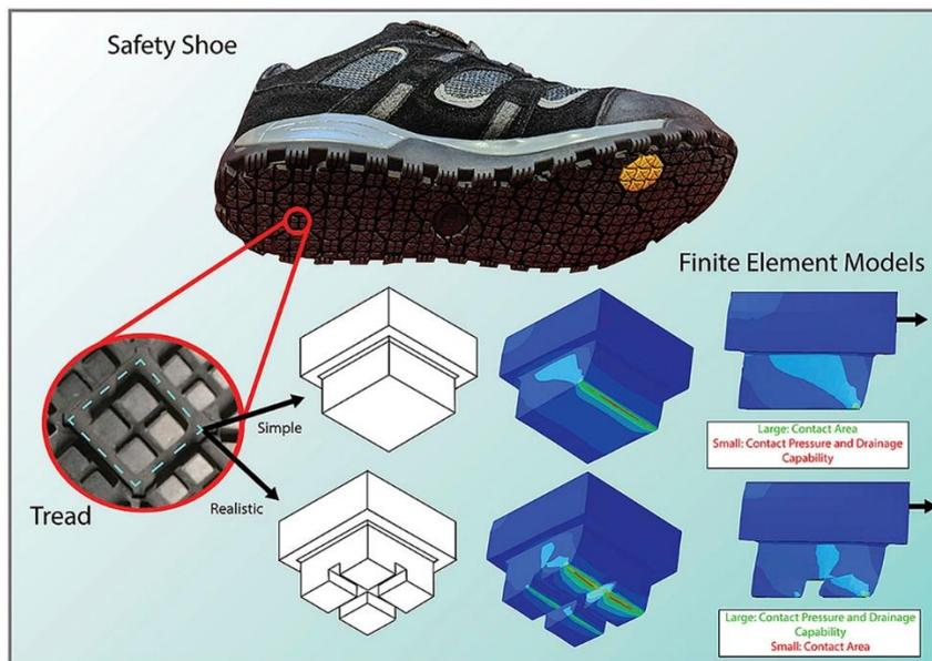
Fig. 7: Virtual testing of footwear outsole.
