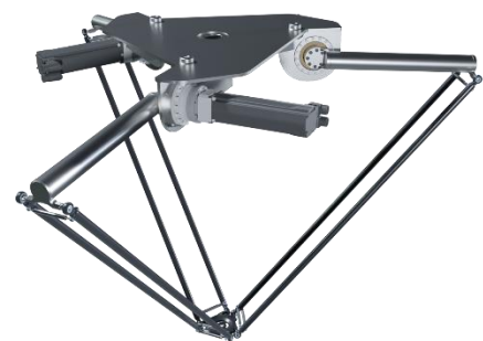
Fig. 4: Robot Delta © PFI
