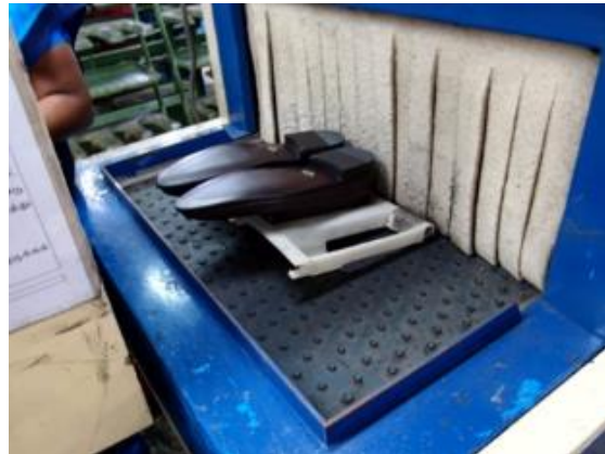
Fig. 39: Solution how to increase the stream of cold on sole © PFI
