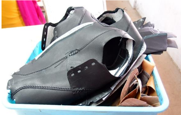
Fig. 9: Random position of part increase searching time © PFI
