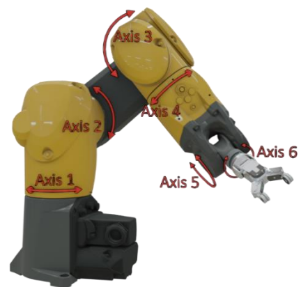
Fig. 2: 6-axis robot with gripper © PFI
