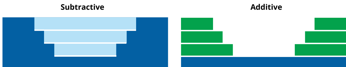
Fig. 7: left: subtractive process (dark blue: desired Part, light blue: removed material) | right: additive process (dark blue: base layer, green: added up layers) © PFI
