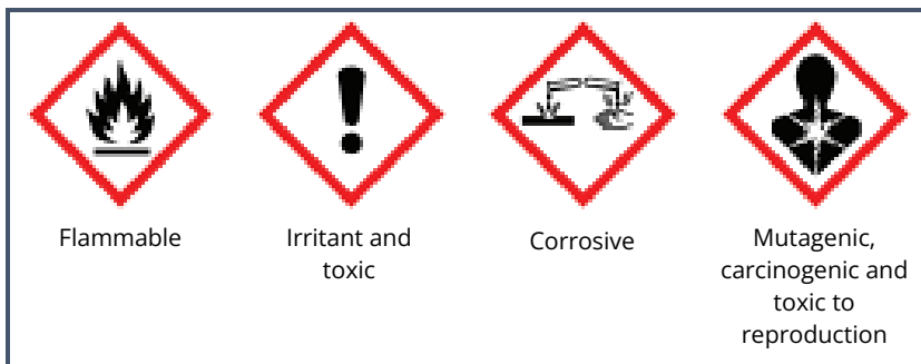
Fig. 12: Chemical hazards - symbology
